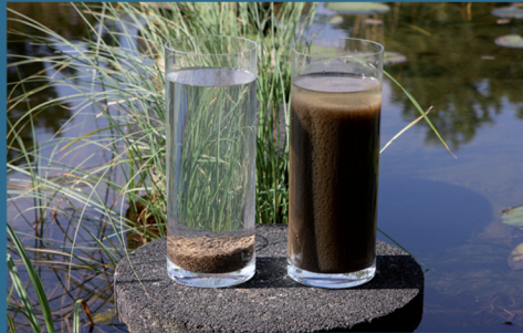
Biomasa de Nereda® (izda.) y lodos residuales activados (dcha.) tras sedimentar durante tan sólo 5 minutos Nereda® biomass (left) and activated sludge (right) after only 5 minutes of settling
