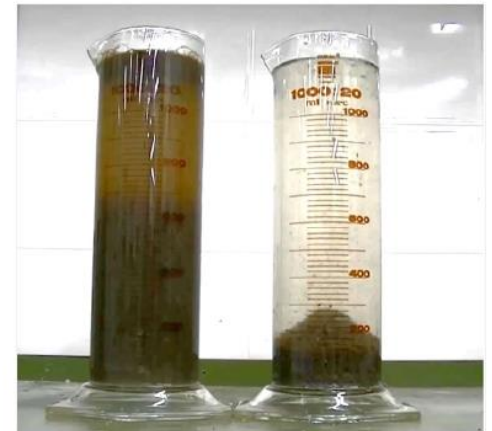
Shock addition of 5,000 ppm NaCl: activated sludge vs. AGS after 5 min settling
